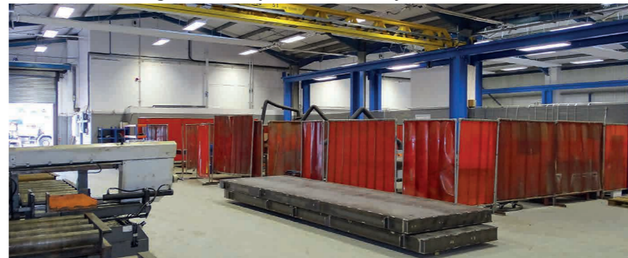
Inside the manufacturing area the workspace is divided into bays with overhead cranes.
