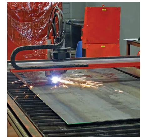
New plasma cutter increases speed and precision
